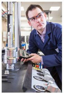
Set-up of a servo-hydraulic fatigue test station © *Jacobs*
